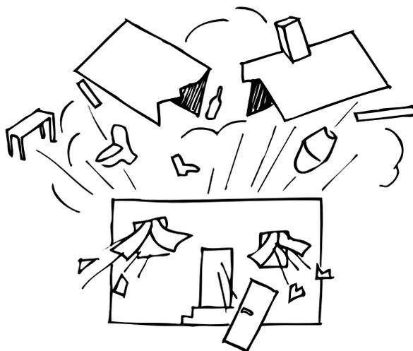
**Explosions** have also occurred. This is nearly always when mixing chemical mash comprising ethyl acetate and sodium hydroxide. Alcohol in gaseous form (the mixture gets hot) spreads into the air. The gas formation is ignited by an open flame or a spark, such as from a thermostat.
