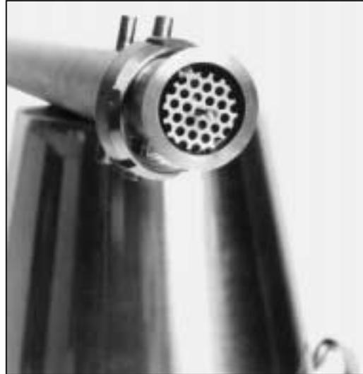
A small stainless strip is welded across the base of the column, onto which is welded a small stainless steel set screw. The perforated plate is then attached to this.
